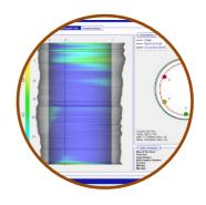
Thermal Integrity Profiling (TIP)
