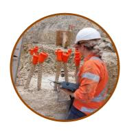
Low Strain Integrity Testing (PIT)
