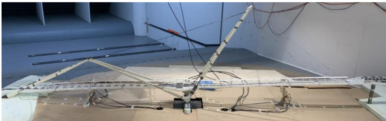
Figure 19 Aeroelastic wind tunnel model
