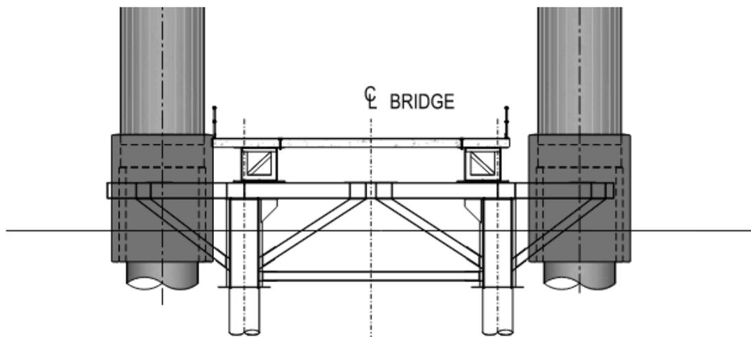
The centrelines of the box girders were therefore positioned a constant transverse distance apart of 14.00m for the 25.15m wide portion of the deck and 14.43m apart for the 29.15m wider section of the deck at each pier. The 10m wide temporary bridge was aligned between the piers and below the inner cantilevers of the box girders.
