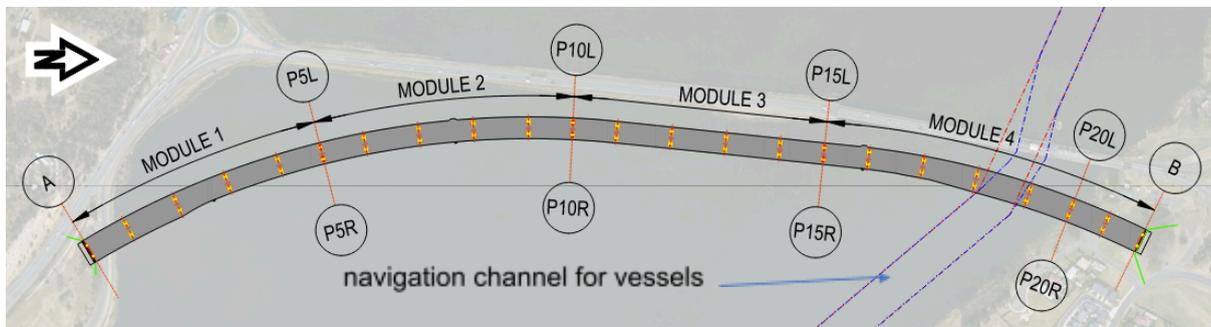
The bridge deck varies in width being typically 25.15m wide, to accommodate two lanes of traffic with 2.0m outside shoulders in each direction along the centre sections, but flares to 29.15m wide for an additional lane to allow for the Southbound exit and entry ramp merges. There is also a 3.00m wide shared user path (SUP) along the western side of the bridge deck. The bridge has a constant 2.2% crossfall on the SUP and 3% cross fall on carriageway towards the eastern side of the bridge.
