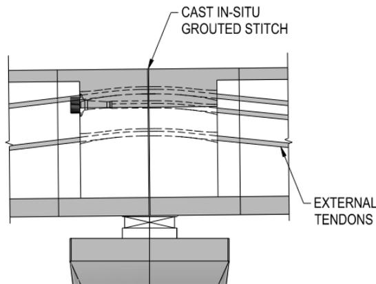
Each expansion joint pier segment is 2m long and has a 1.5m long internal diaphragm wall. The weight of this pier segment is around 84 tonnes. The diaphragm wall of this segment is used to anchor the 2 x 4 No. 6-31 external tendons as well as accommodating the bearing forces from both the permanent bearings and also the temporary jacking points used during construction
