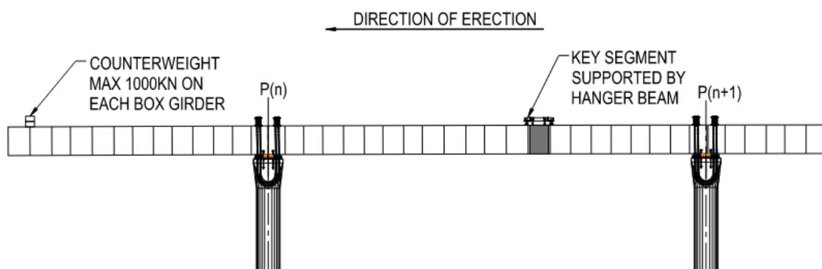
It is worth noting that when it comes to soil structure interaction calculations such as these, the observed deflections are in the author’s experience always less than calculations using the engineering properties of the soil would predict. This was also the case for this bridge. It was for this reason a permissible range of offsets for the counterweight was provided so that MCD could move the counterweights as required to get a balancing deflection.
