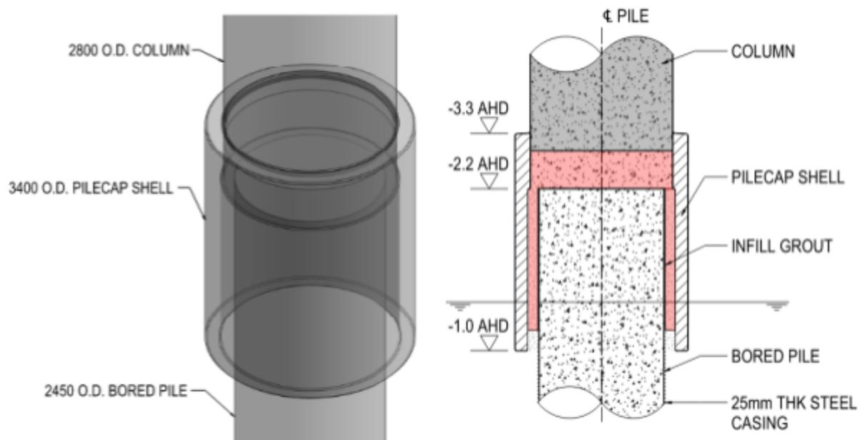
The shell was concreted to the top of the pile using a 750mm thick slab that was poured in-situ, with the pile reinforcement passing through and up into the main body of the pier. The gap below this slab between the annulus and pile, notionally 160mm wide but varied depending upon the final position of the pile, was filled with concrete to protect the steel casing of the pile from corroding in the tidal zone.
