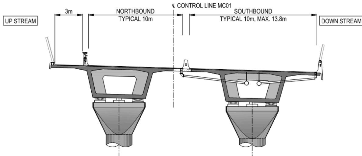
The bridge was designed to allow for the future installation of an underslung services gantry underneath the soffit in the centre of the bridge. The gantry will accommodate 1 no 400mm diameter sewer main, 2 nos 300mm diameter water mains and a 1.2m wide maintenance accessway.
