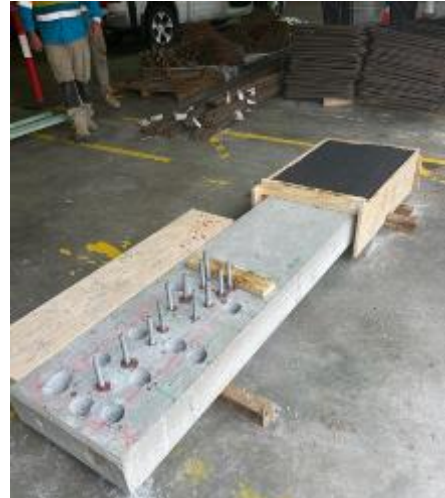
Figure 3 Scanning trials and anchor testing
