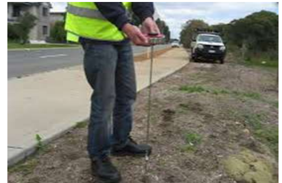
Hand-held Shear Vane Test
