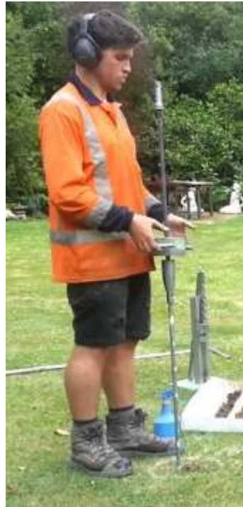
Scala Penetrometer Test
