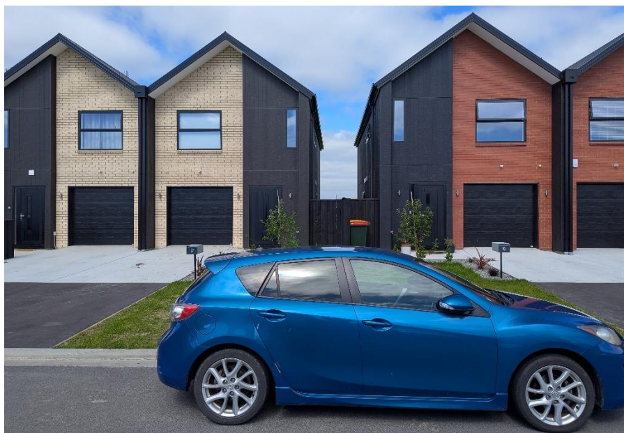
Figure 3 – Example of closely spaced driveways reducing on-street parking capacity (Source: SDC)
