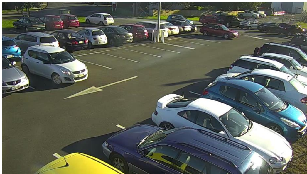
Figure 3: Analysis of CCTV footage was a cost-effective and innovative way of determining park and ride parking occupancy levels during the morning peak
