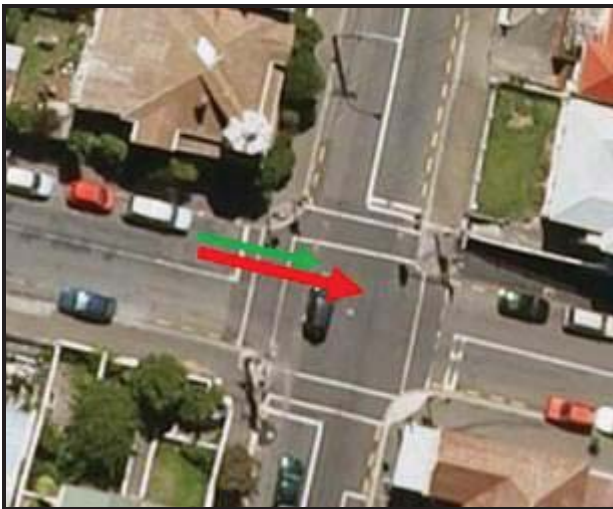
C3 Intersection/Access Approach side-swipe
