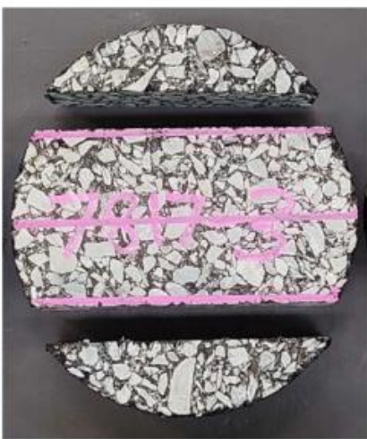
Cutting the top, bottom, and sides of each specimen
