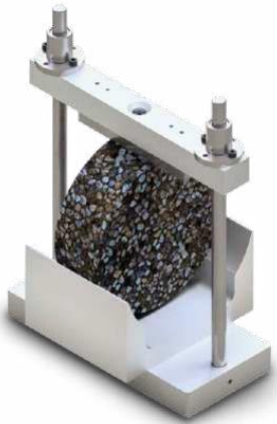
Rapid Shear Rutting Test (IDEAL-RT) (surrogate for Hamburg)
