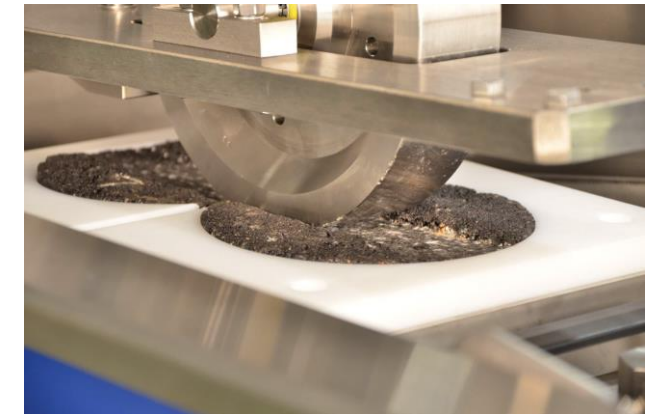
Hamburg Wheel-Track Test in Air or Water
