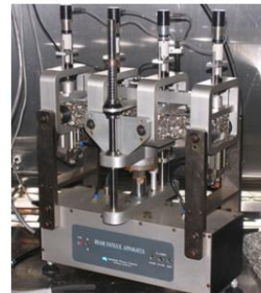
FLEXURAL BENDING BEAM FATIGUE
