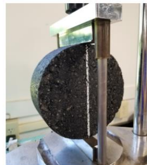
INDIRECT TENSILE ASPHALT CRACKING TEST (IDEAL-CT)
