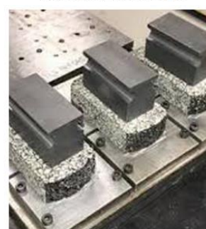
IDT CREEP COMPLIANCE AND STRENGTH TEST
