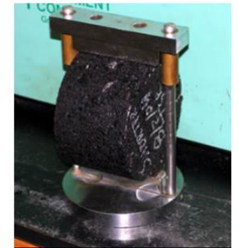
TENSILE STRENGTH RATIO
