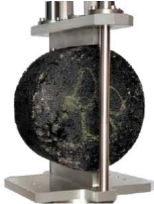
Indirect Tensile Asphalt Cracking Test (IDEAL-CT) (surrogate for I-FIT)
