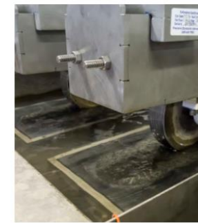
HAMBURG WHEEL- TRACKING TEST
