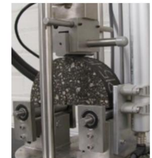
ILLINOIS FLEXIBILITY INDEX TEST (I-FIT)
