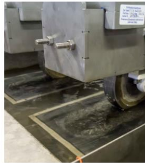
HAMBURG WHEEL- TRACKING TEST
