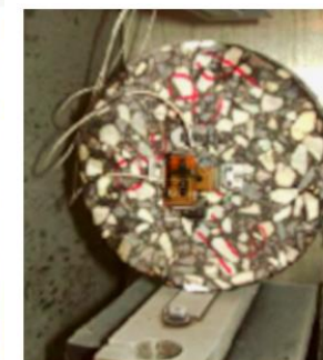
IDT CREEP COMPLIANCE AND STRENGTH TEST
