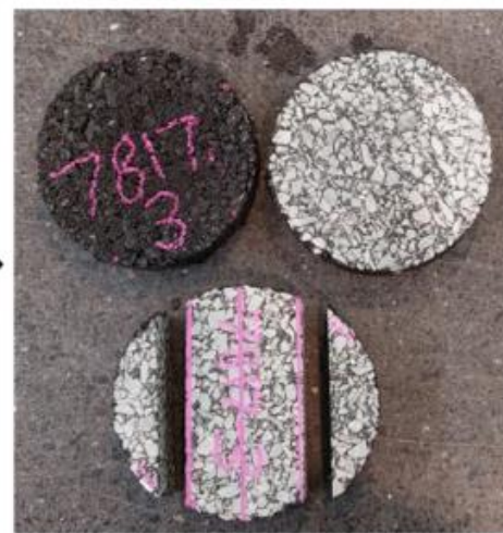
Cutting the top, bottom, and sides of each specimen
