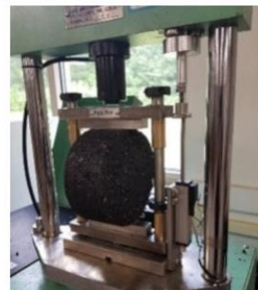
HIGH TEMPERATURE INDIRECT TENSION (HT-IDT)
