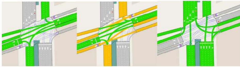
Figure 6: Signal groups for a single lane on each side, separated cycleway (cycleway turns in yellow)
