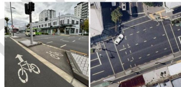
Figure 25: Separator gap waiting space for cyclist turning right on T-Intersection of Karangahape Rd and Howe St
