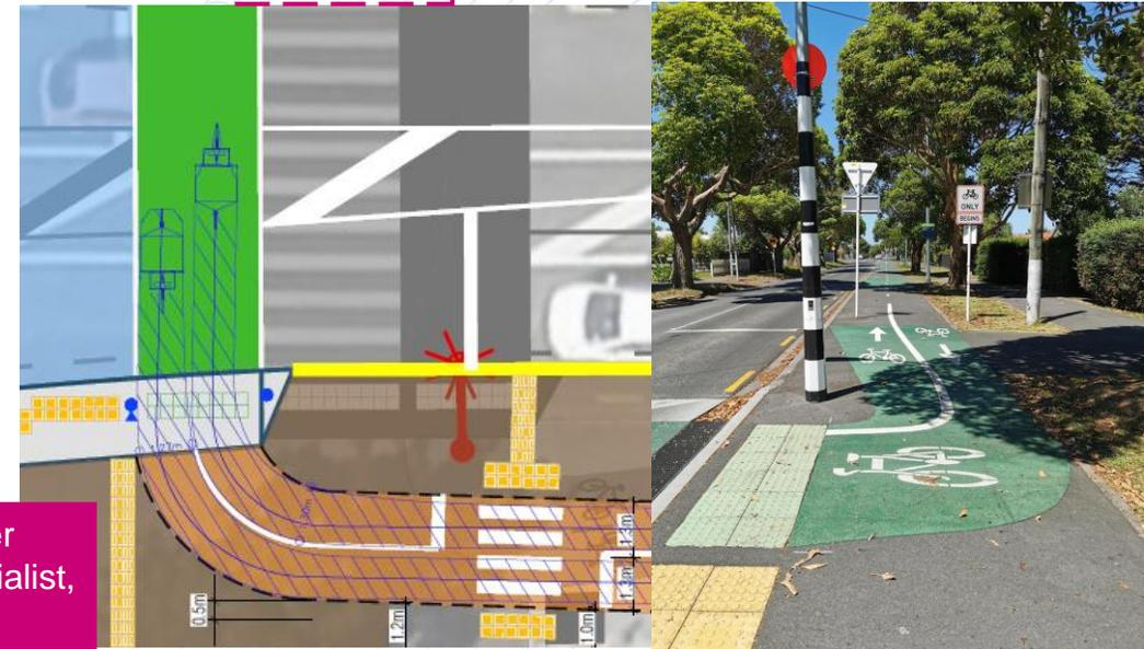
Minimum for constrained environment - with maximum length.
