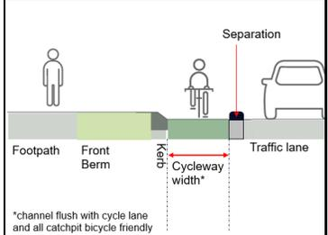
PN04-3 Diagram 2: Cycleway Width in a constrained environment
