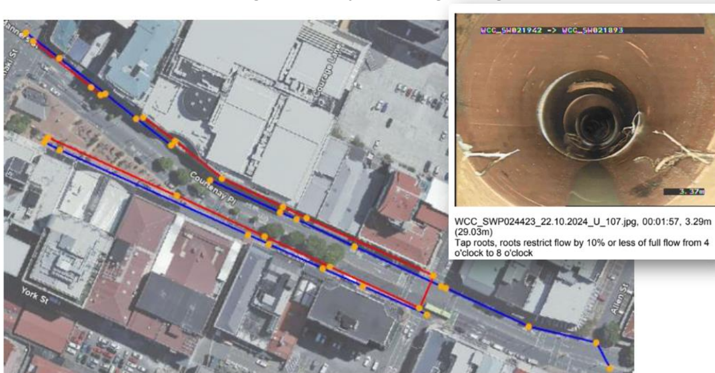
Figure 3. 58 - 134 Courtenay Place WW and SW Renewals (WW - Red, SW - blue, Manholes - orange)
