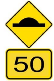
Figure 5: Warning signs at ramp locations
