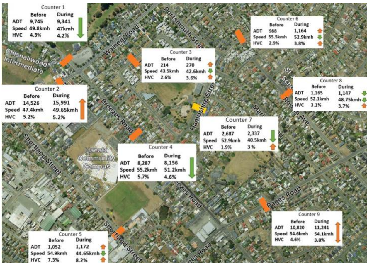
Figure 7: Number of motorists, operating speeds and number of heavy vehicles on streets before and after safety interventions were added. Data sourced from pneumatic tubes.
