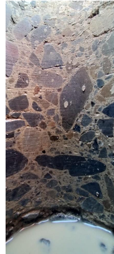
Typical Core using new rolling pattern (Plateau using Backscatter, DT100 and DT200)
