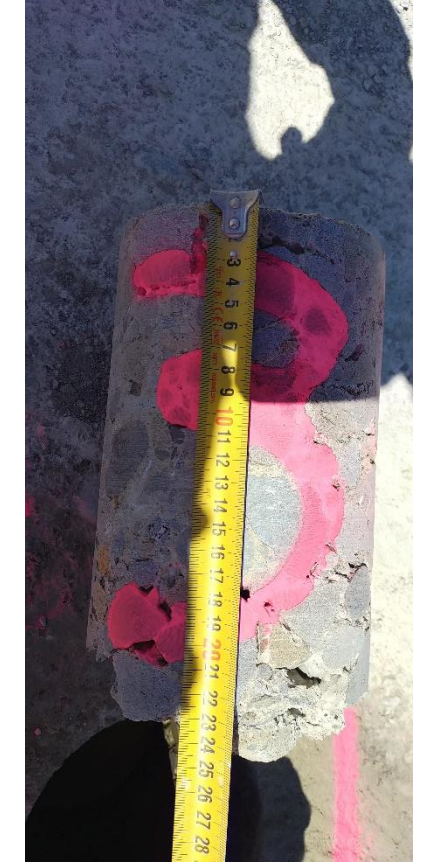
Typical Core using new rolling pattern (Plateau using Backscatter, DT100 and DT200)
