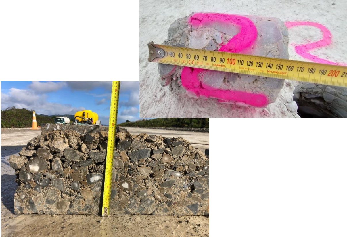
Original rolling pattern (Plateau using Backscatter) – Note conforming Density check using Backscatter
