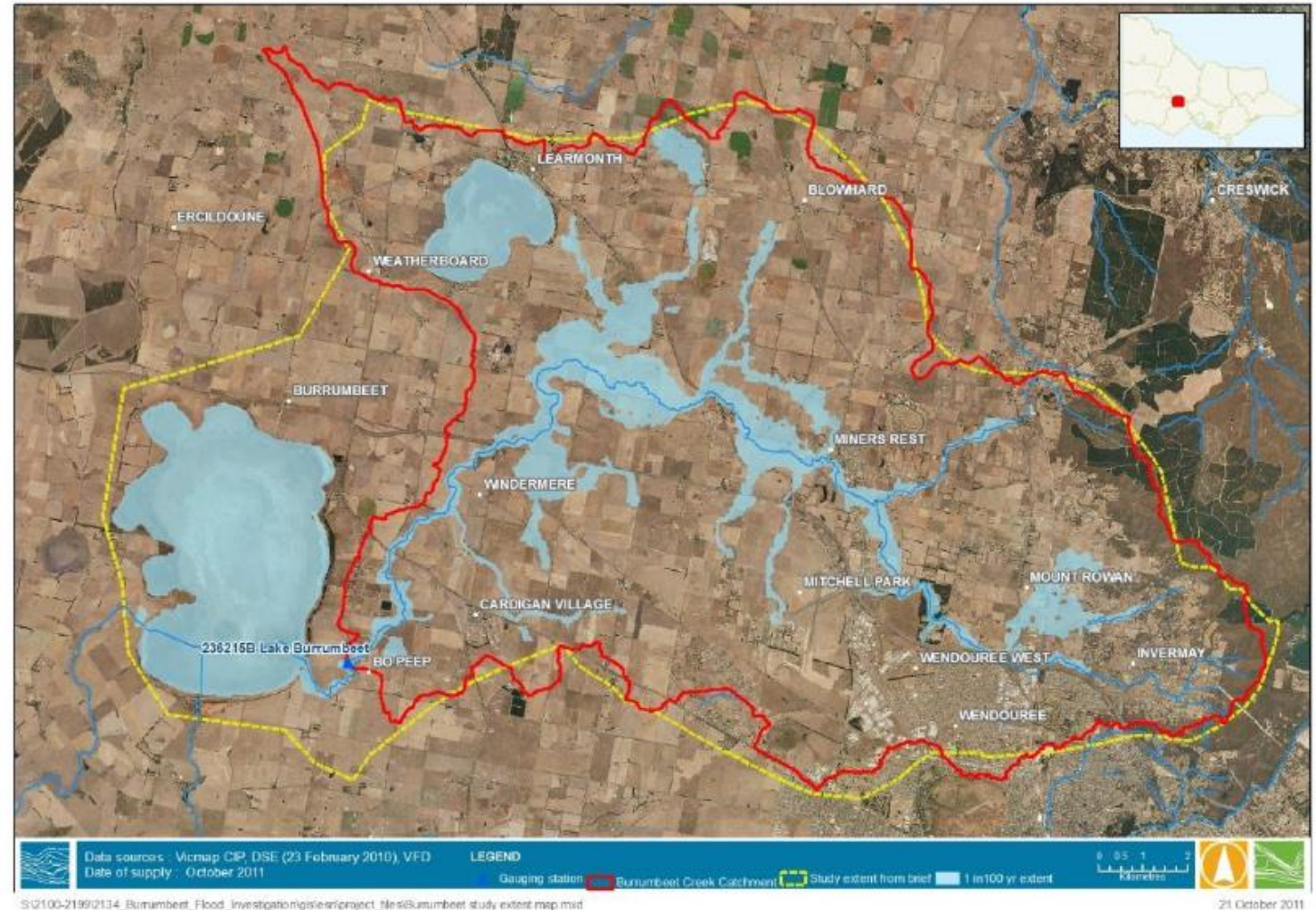
Figure 1-1 Study area showing Burrumbeet Creek gauge catchment and previously modelled 100 year ARI flood extent (Lawson and Treloar, 2003)
