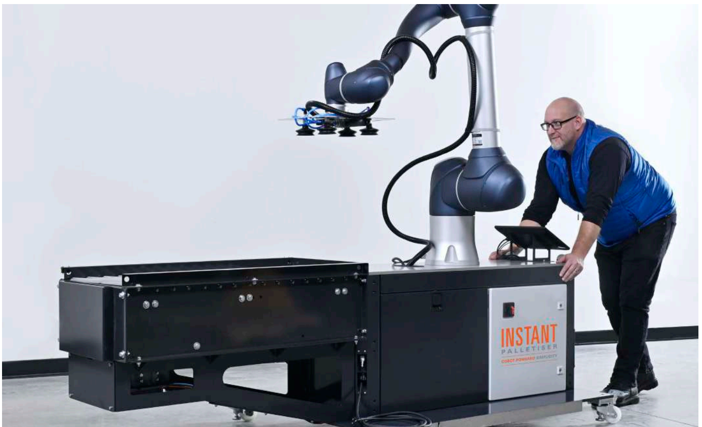
Mobile cobot palletising: Palletise to two locations simultaneously, up to 30kg payload
