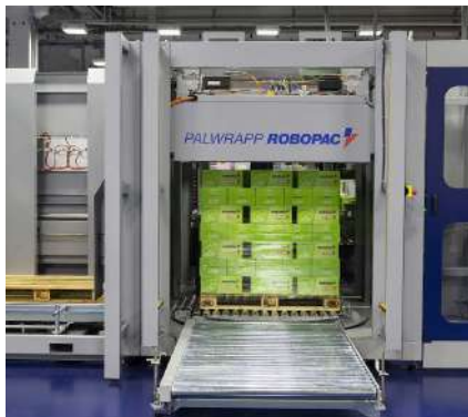
Mechanical PALWRAPP with built-in stretch wrapping
