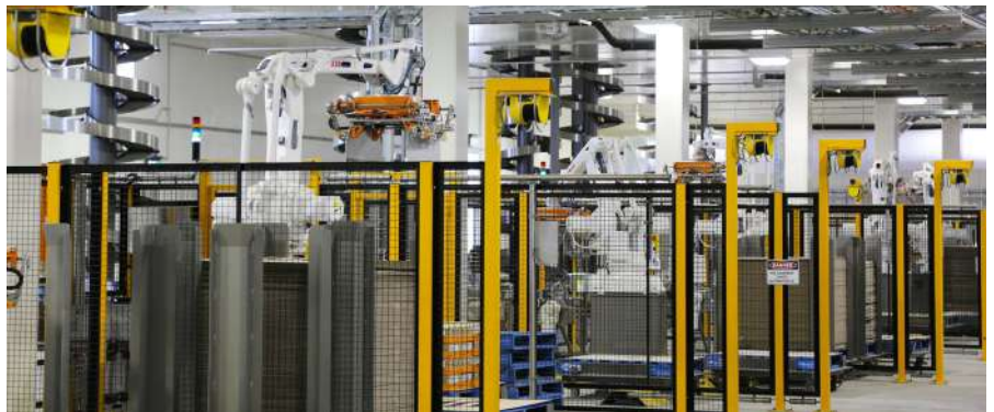
8-line centralised medium-speed pick and place
