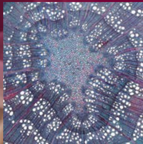
Oak wood fiber under the microscope.
