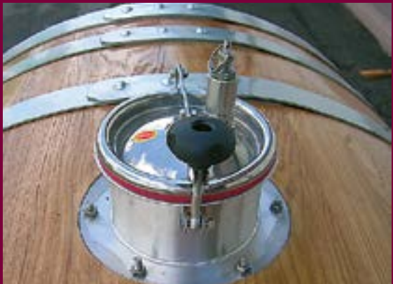
Stainless steel 18/10 AISI 316 bung-hole stopper 16-22 cm diameter, 9 cm high, complete with pressure valve in steel or moplen. Total drainage pipe in stainless steel.
