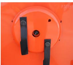
10 Gauge stump jumper allows cutter to slide over obstructions protecting the gearbox output shaft.
