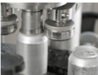
**Pre-threaded caps:** suitable for the application of the pre-treated caps on glass or plastic bottles. Application is done by picking the cap from the feeding mechanism, with the capping head chuck, placing and screwing it on the bottle with desired torque, called pick and place method.
