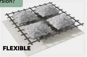
FLEXIBLE - The flexible version is more pliable due to the excess concrete having been removed from between the shapes, this exposes the geogrid openings which allows water to filter through, captures sediment, and vegetation can grow through the spaces. The less rigid nature of the mat makes it more pliable in three directions.
