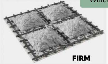
FIRM—This version is "firm" because it retains the excess concrete between the concrete shapes. The polyester geogrid is less exposed and the whole mat is more rigid. The mat retains its permeable qualities, however the non-woven underlay is attached by excess concrete to the mat, which will further inhibit growth of vegetation coming through the mat. The more rigid nature of the firm mat makes it less pliable, its flexibility is in two directions.
