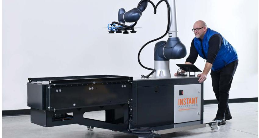
Or it can be configured to stack two different SKUs simultaneously. It can even insert slip sheets on the base or in between layers.
