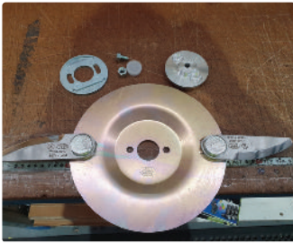
DISKS WITH FLAIL BLADES FOR TOPPING VINES POST HARVEST
