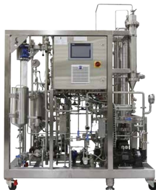
Pictured: Flavourtech's standard SCC100. The new SCC100-W will come with a separate control panel located outside any hazardous area.
