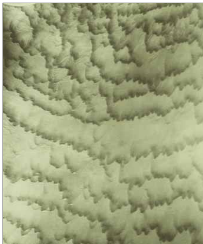
High speed photo of the liquid film on the heat transfer surface of the Centritherm evaporator. The film is only 0.1 mm thick and crosses the surface in about 1 second resulting in a well defined residence time. The photo also shows substantial agitation in the liquid film, one of the factors that contribute to its high efficiency.
