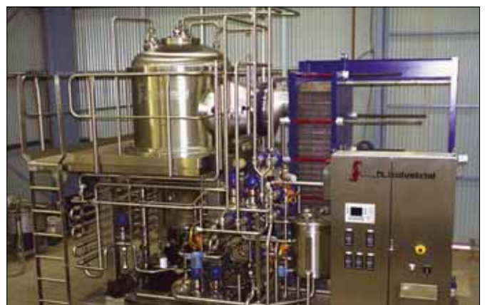
CT-9 for tea and coffee extract installed 2003
