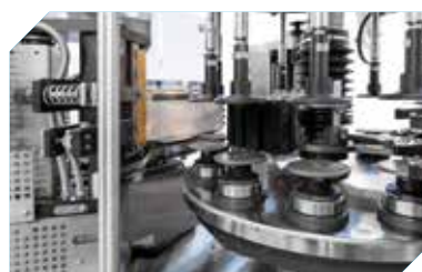
Label magazine and roll for glue application on the label overlap.
