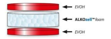
Combined with Meyer Seals® ALKOzell™ closed-cell foam. ALKOvin™ EVOH offers a sealing system with excellent protection against oxygen ingress. ALKOvin™ EVOH guarantees a controlled low level of oxygen transmission. This sealing liner is free from chlorinated hydrocarbons (PVDC).
