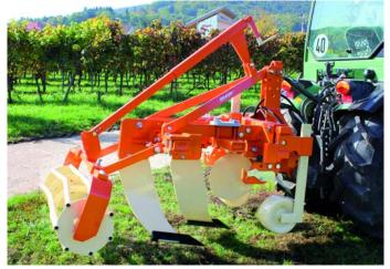
Cultivator *Vario* equipped as para-plough with swivelling coulter discs, stabilising wheels and tube roller
