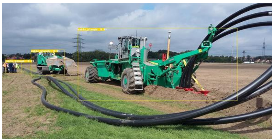
Figure 5: Output of the YOLO v4 object detector: objects location in the form of bounding boxes and classification.
