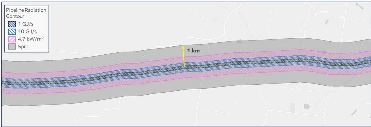
**Figure 3:** Pipeline radiation contour example showing area of interest either side of pipeline
