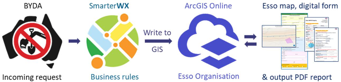
**Figure 8:** The (simplified) data flow originating with a BYDA request which is then processed with SmarterWX and pushed to Esso's ArcGIS Online Organisation where it is pulled into a digital form
