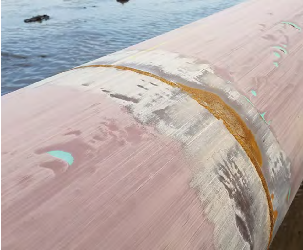
Failure of Two-Part Epoxy
