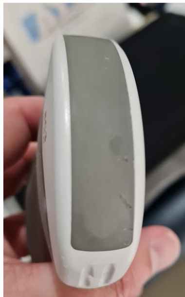
Matching layer damage
