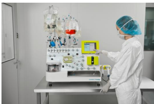
A $150,000 instrument being tested in gene-therapy studies of cancer. It automatically adds a new gene to a person's blood cells.
