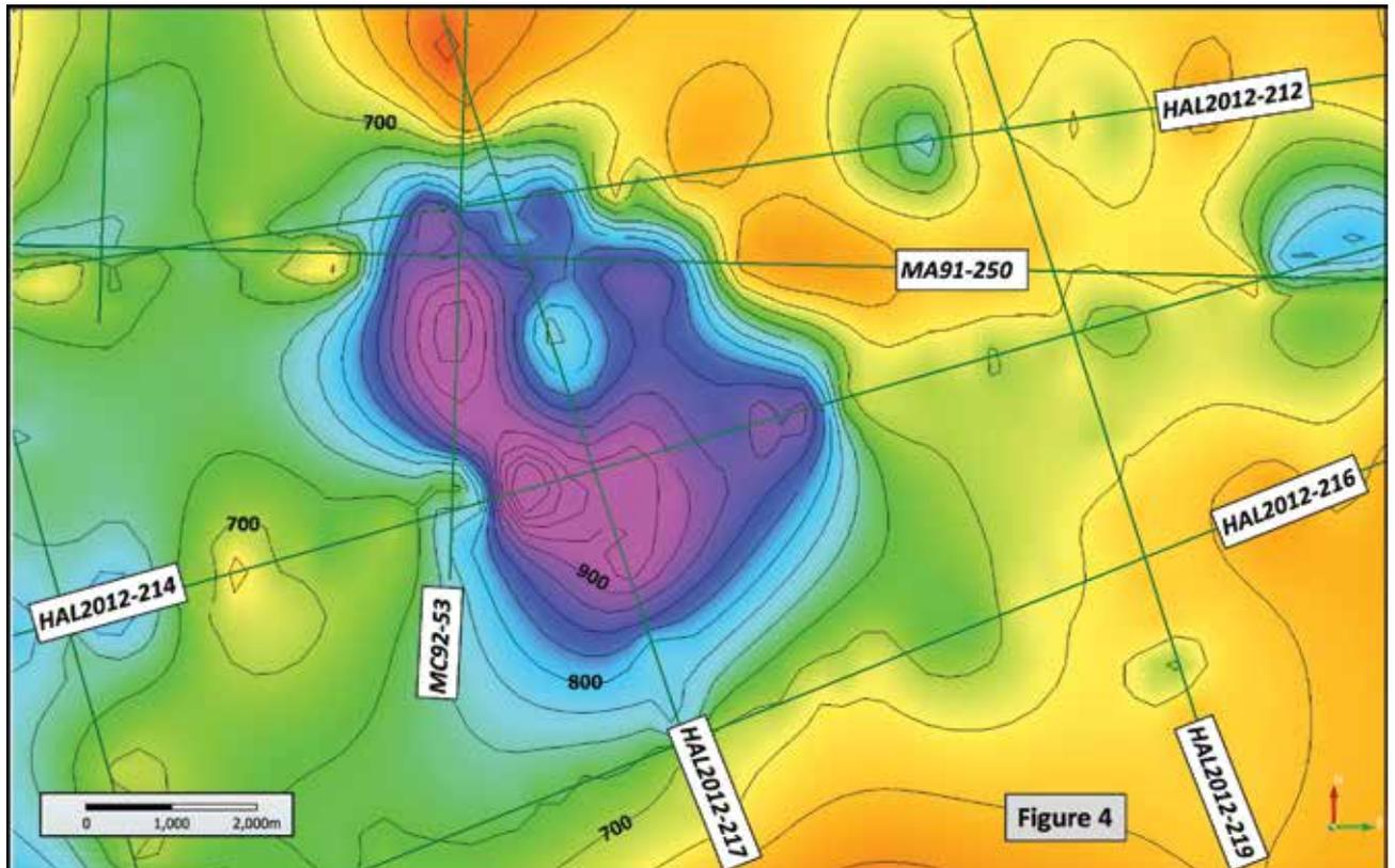
Figure 4: Top Jamison sandstone subsea depth map based on PSDM seismic. Depth of the crater ~ 250 m. Fault pattern not shown, 3D seismic required.
