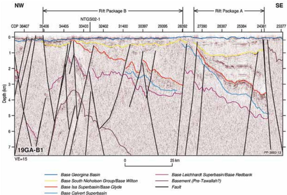
Figure 3: Interpreted seismic profile of the Beetaloo-McArthur domain
