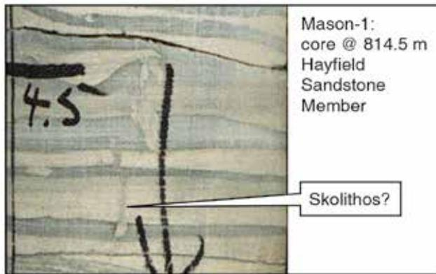
Figure 6. Possible *Skolithos* trace in interbedded shallow marine strata of the Hayfield Sandstone Member in Mason-1 at 814.5 m. Note also possible horizontal *Planolites*-like trace (white oval in grey siltstone). Arrow points towards the base of the core. *Planolites* is unlined and having an infill different than the host rock (Pemberton and Frey, 1982).
