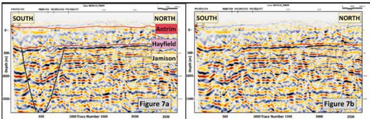
Figure 7a, b: PSDM line MC92-53 interpreted (left) and not interpreted (right). PSDM processing to 2000m with black indicating an increase in acoustic impedance. Note smooth Antrim Volcanic section and undisturbed Hayfield section either side of the fault bounded low.
