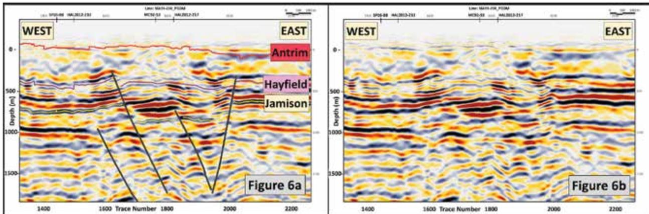
Figure 6a, b: PSDM line MA91-250 interpreted (left) and not interpreted (right). Line location in Figure 4. Line inter-sections at top. PSDM processing to 2000 m. Note smooth Antrim volcanic section and thickened Hayfield. Black is an increase in acoustic impedance.
