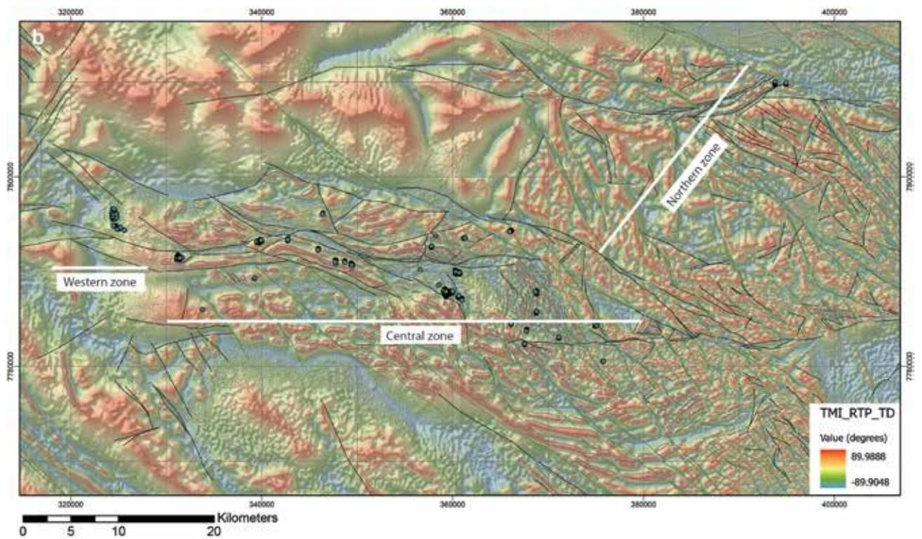
Figure 2: (b) Total magnetic intensity, reduced-to-pole tilt derivative image.
