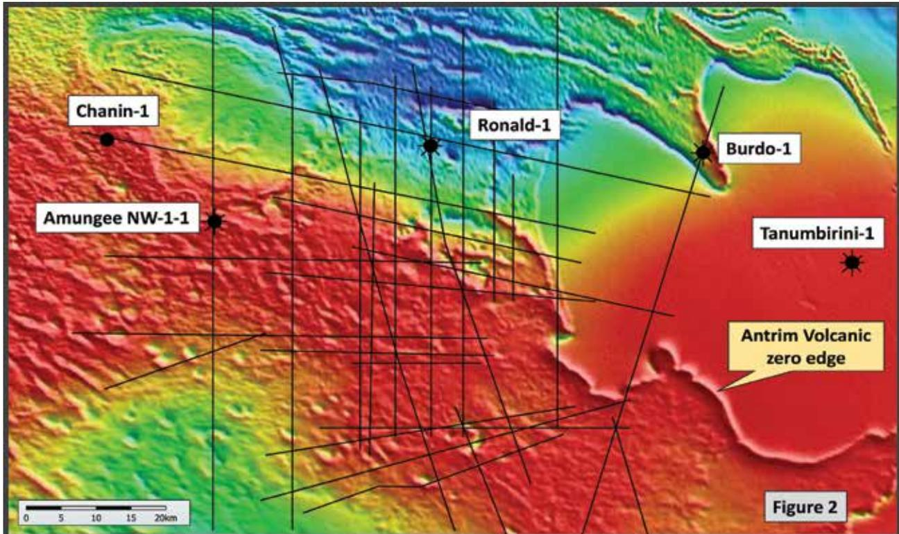
Figure 2: Total Magnetic Intensity (TMI) with Pre-Stack Depth Migrated (PDSM) seismic and wells.
