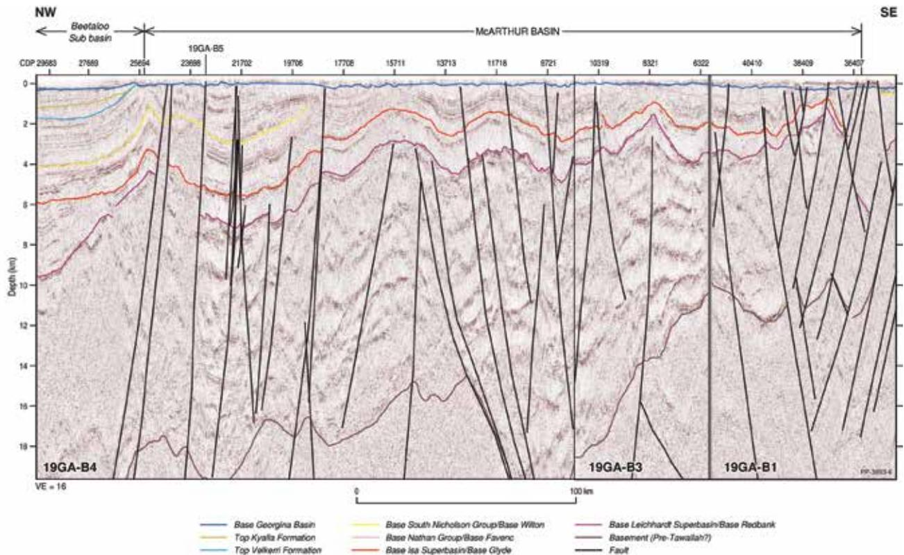
Figure 4: Interpreted seismic profile of the Beetaloo-McArthur domain.
