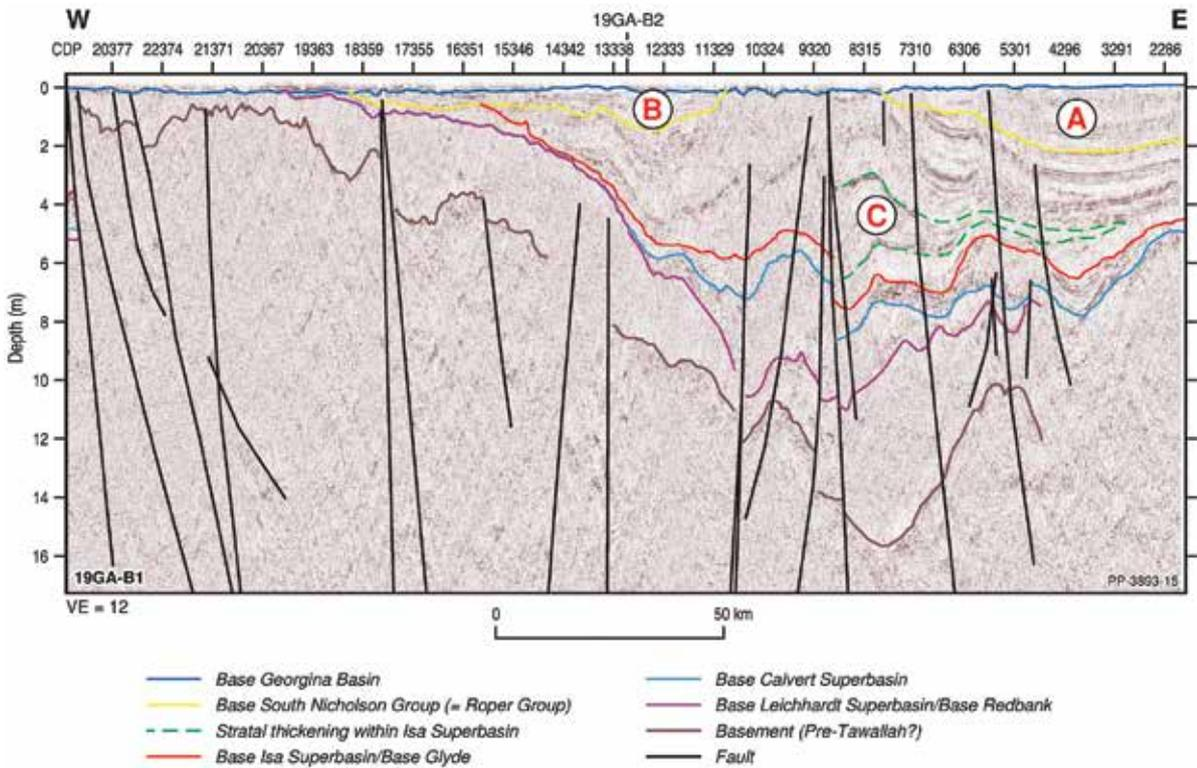
Figure 2: Seismic profile of the Carrara domain incorporating the south western part of the Carrara Sub-basin to a shoulder of metamorphic basement. Labels 'A' and 'B' denote the structural remnants of the South Nicholson Group and 'C' denotes an area of syn-depositional River extension.
