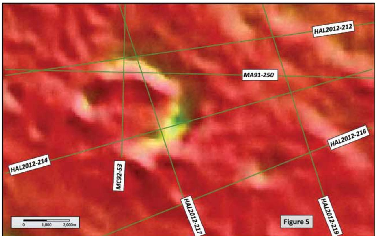
Figure 5: Detailed TMI image showing coincident anomaly with underlying Jamison structure.
