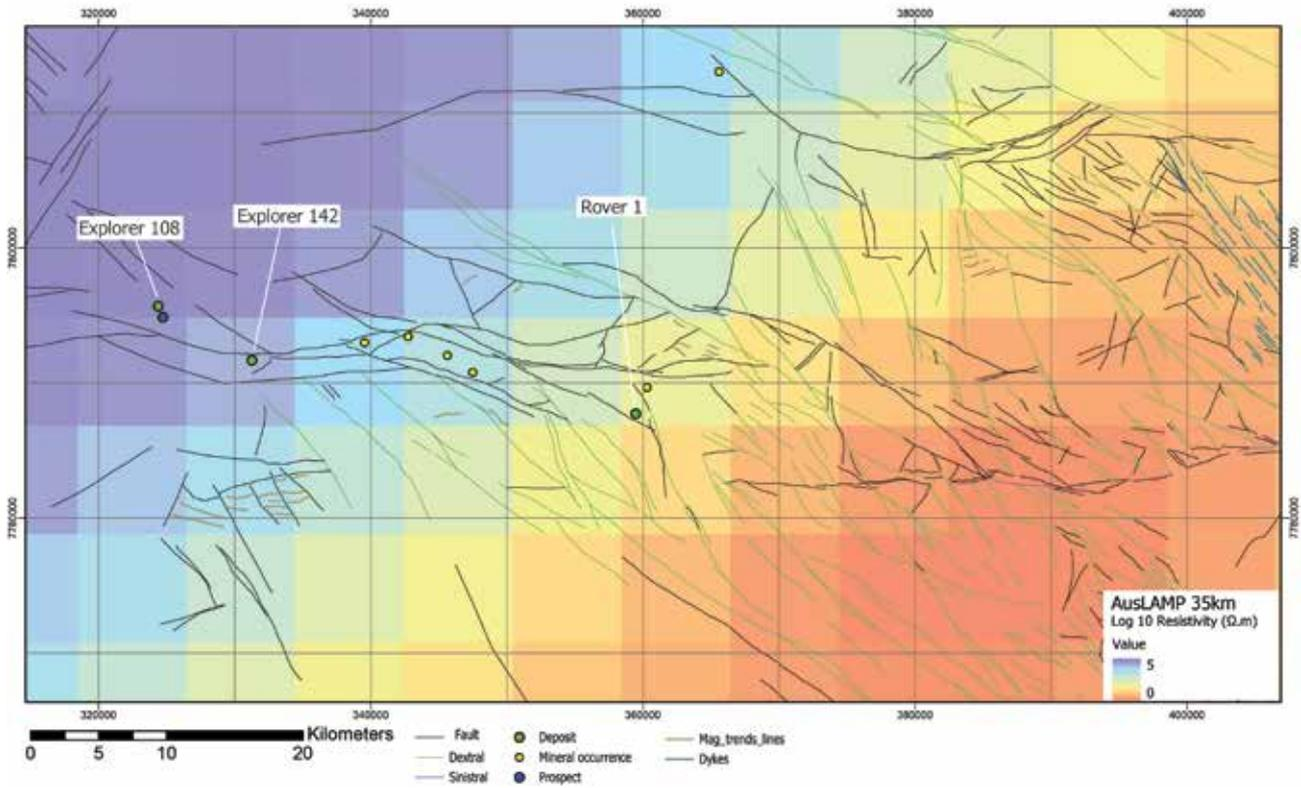
Figure 2: (c) Resistivity map of the Rover field with interpreted zones.
